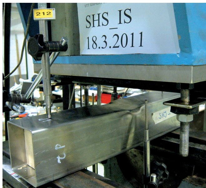
Figure 6 Failure of a SHS beam by web crippling
